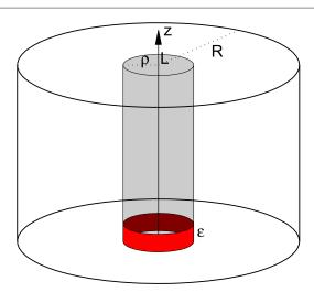
**Figure 1.** Schematic presentation of the cylindrical domain  $\Omega$  between two cylinders of radii  $\rho$  and R, capped by planes at z=0 and z=L. The target region is a red annulus of radius  $\rho$  and height  $\epsilon$ .
