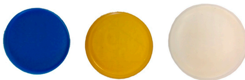
Figure 3. Photograph of ionogels (IGs) used in this study. IGs are based on [\text{Bmim}]_2[\text{CoCl}_4] (left), [\text{Bmim}]_2[\text{CuCl}_4] (middle), [\text{Bmim}]_2[\text{MnCl}_4] (right). The ionic liquid (IL) loading is 20%.
