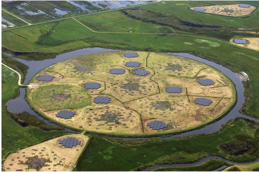
Figure 4.2: The most central LOFAR core stations in the Netherlands which are used for solar imaging observations. Each core station consists of one low- and two high-band antenna fields. The six stations on the island are called the Superterp.
