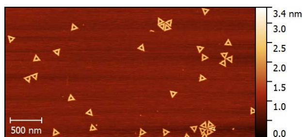
Figure S 1. Typical AFM image of triangularly shaped DNA origami structures on freshly cleaved mica.
