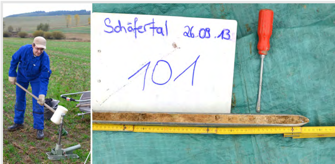
Fig. 1.1: One of 30 locations during a soil sampling campaign in the Schäfertal . An auger is pushed up to 80 cm into the soil and subsequently pulled out. The soil colors and texture reveal insights into the composition of the vertical soil profile.
