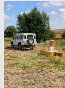
Fig. 11: Surveying spatial patterns of neutrons (inside rover) and natural gamma rays (trailing sled) in the Schäfertal .
