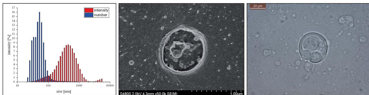
Fig. 1 Analysis of the turbid vesicle template phase via DLS intensity and number plot (left), the corresponding Cryo-SEM micrograph (center), and the image of light microscopy (right).
