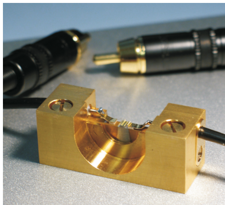
Figure 7.19: Picture of the tapered amplifier with separate contacts for ridge and tapered section on the high power heat sink. (Picture copyrighted by m2k-laser GmbH).
