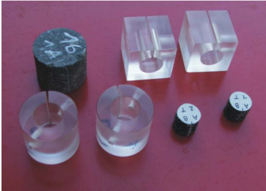
Figure 2.1. Two mini-samples of 12 mm diameter with four non-magnetic adapters. Cylindrical adapters allow for measuring mini-samples in equipment that is designed for standard-size samples such as the JR5/JR6 spinner magnetometers, cubic adapters e.g. for measurements on the long-core 2G system. A standard-size sample with 25 mm diameter is shown for comparison.
