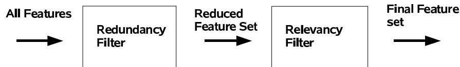
Figure 2.2: Filter approach for unsupervised feature selection after Li et al. (2007).
