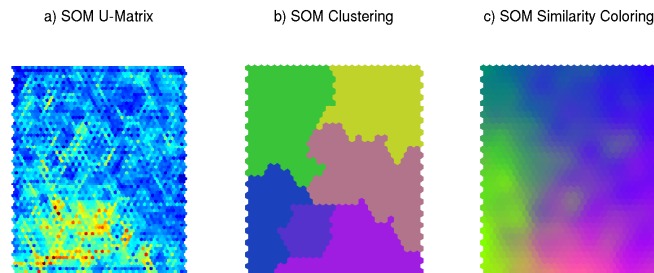
Figure 5.19: U-matrix, best clustering ( k = 6 ), and SOM similarity coloring for earthquake data set (RDO).
