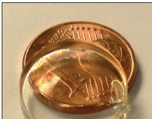
Figure 3.4: Transparency of a LCBS-C 10 silica gel (20 mol% mixture in TEOS)
