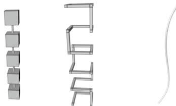
Figure 3.23: Voxel line, grid cell line, smoothed geometry.
