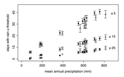
Fig. 3. Comparison of rain pattern in exemplary 30-yr time-series (outline symbols) generated by the ReGen model (Tab. 2) with that of historic rain data (filled symbols; Tab. 1). Error bars indicate 95%-confidence intervals. Thresholds: squares: 5 mm, diamonds: 15 mm, circles: 25 mm.
