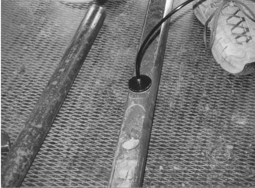
Fig. 5.11. Photograph of the core barrel sampler and the LIF sensor head used for scanning the soil core.
