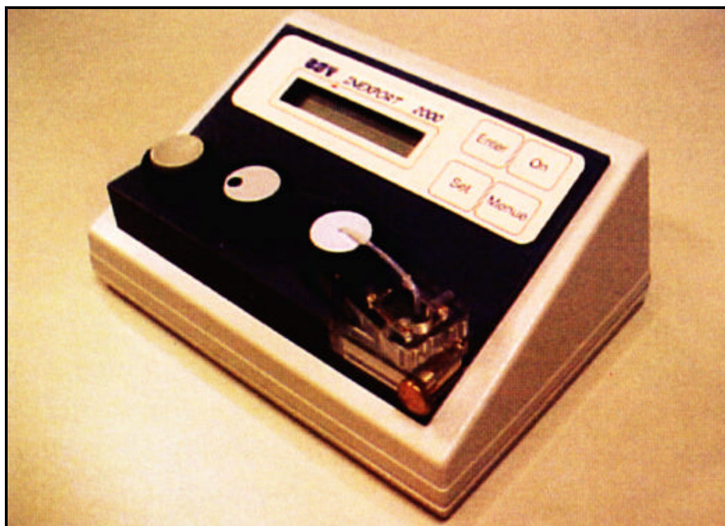
Figure 4.52: Final portable device for on-site analysis of phenolic compounds using a GDH-biosensor.
