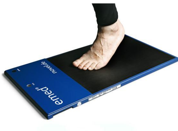
Figure 9: Walking over plantar pressure plate (PEDAR)(left), plantar pressure distribution (parameter: peak pressure, COP) calculated by software Novel, Pedar (right)
