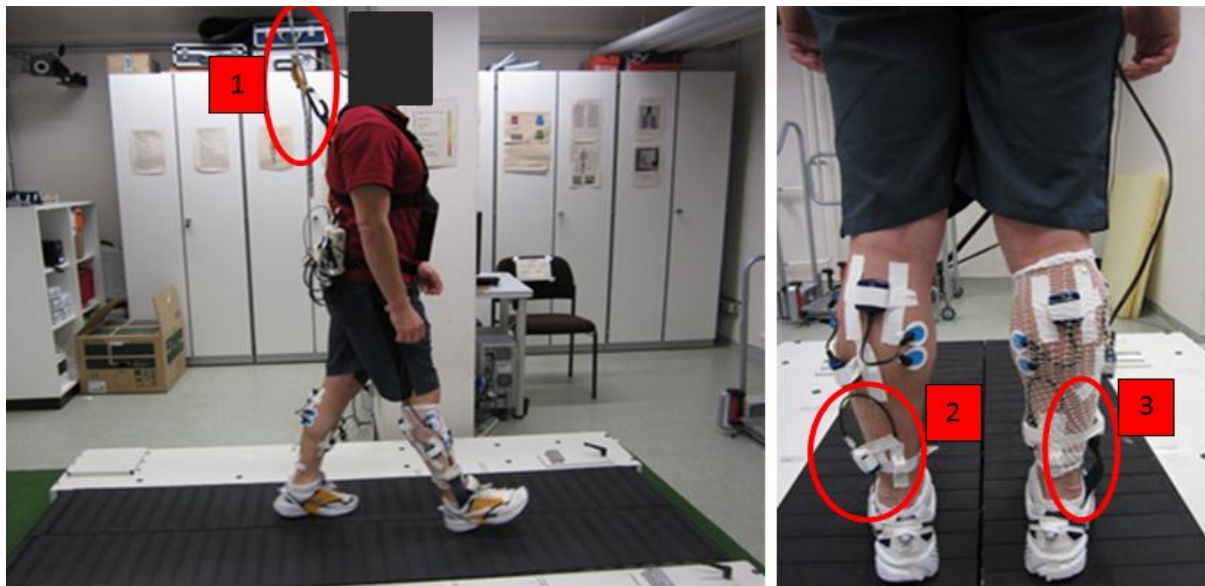
Figure 11: Walking on split-belt treadmill (WOODWAY) with security restraint system connected with the ceiling (red mark 1); in-shoe-sole connected with PEDAR X software at right leg (red mark 3), accelerometer at left leg (red mark 2)
