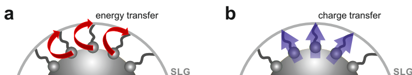
Figure 4.6.: Postulated mechanisms for the fluorescence quenching within graphene covered AuNPs. (a) Energy transfer from excited dye molecules to SLG. (b) Charge transfer from the AuNP to SLG mediated by the DNA coating in between.
