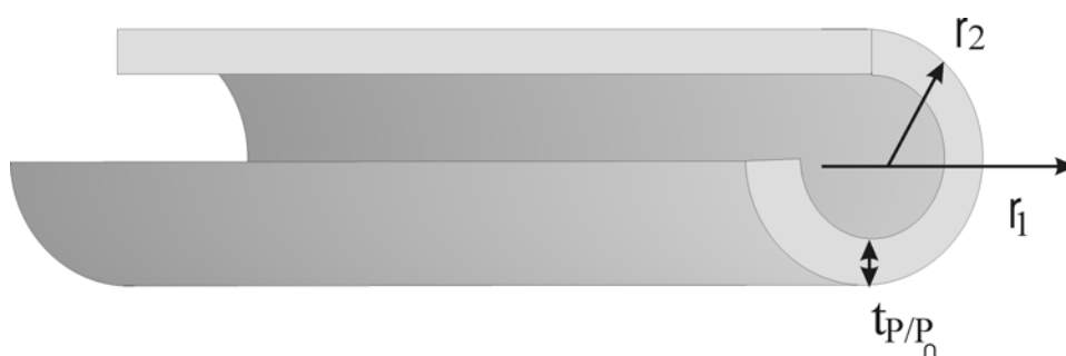
Figure 3.2 Schematic representation of a section through a cylindrical pore with nitrogen molecular monolayer on the pore wall.
