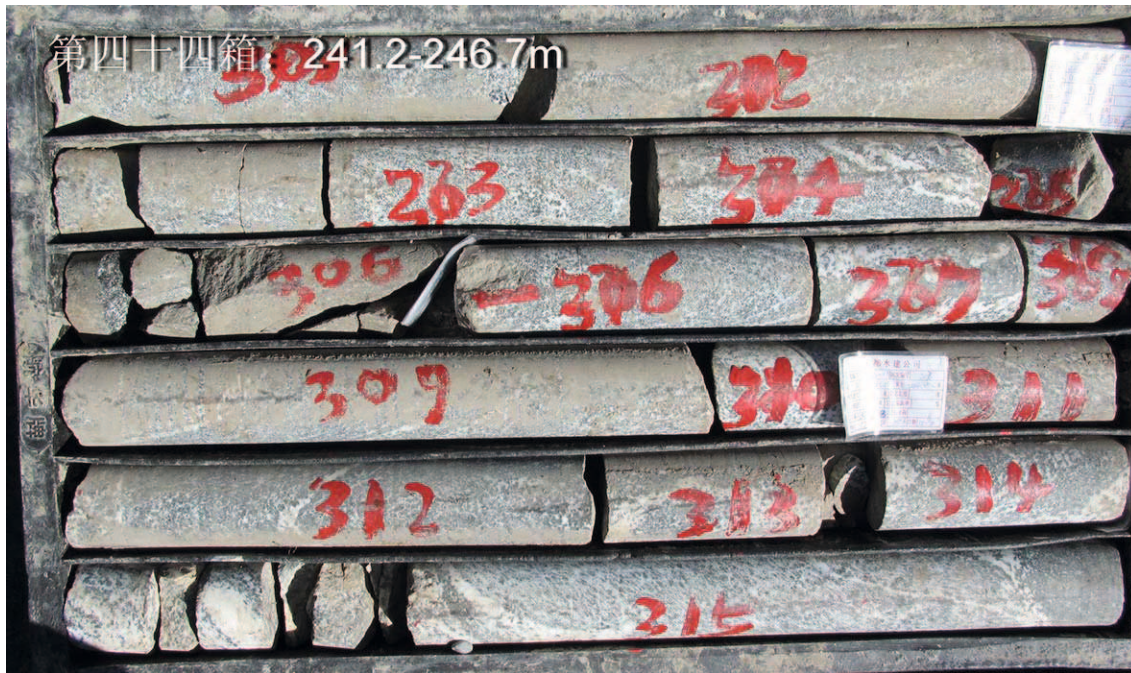
Figure 4.5: Drill core recovered from drilling site #5 at a depth of 241.2–246.7 m. This section consists of gneissic bedrock. The width of the box is ~ 1 m..
