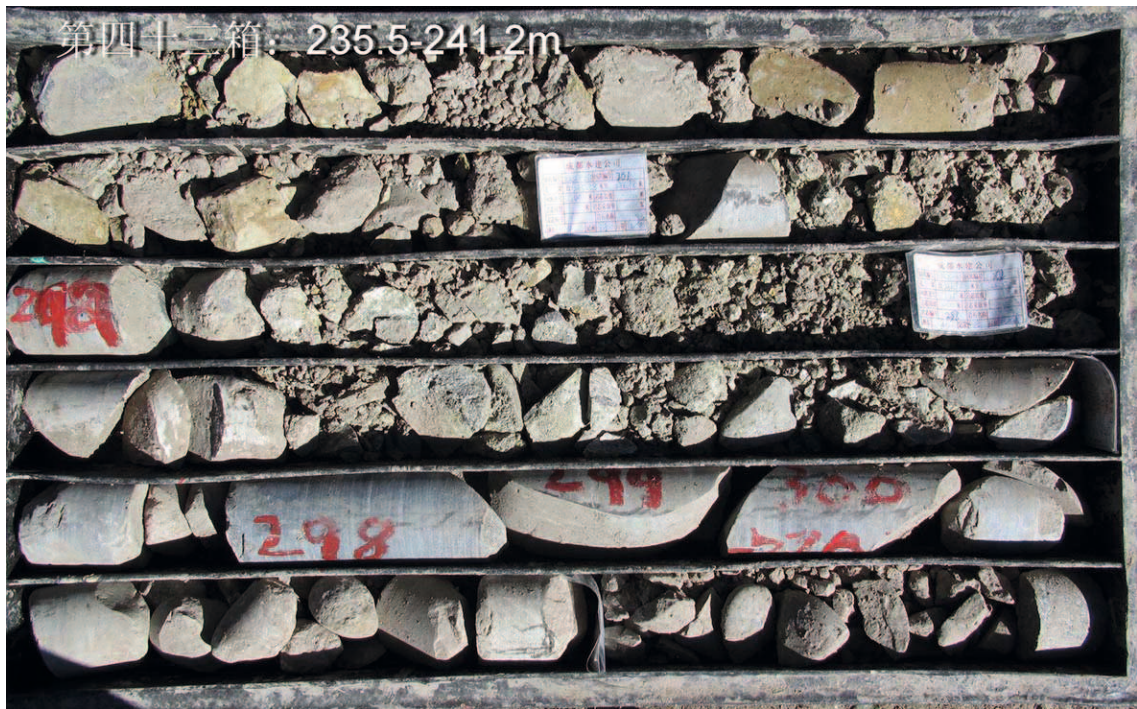
Figure 4.4: Drill core recovered from drilling site #5 at a depth of 235.5–241.2 m. This section consists mainly of unconsolidated sand, gravel, and pebbles. Rounded pebbles near the bottom indicate fluvial transport. These deposits constitute the base of the valley fill at this site. The width of the box is ~ 1 m.
