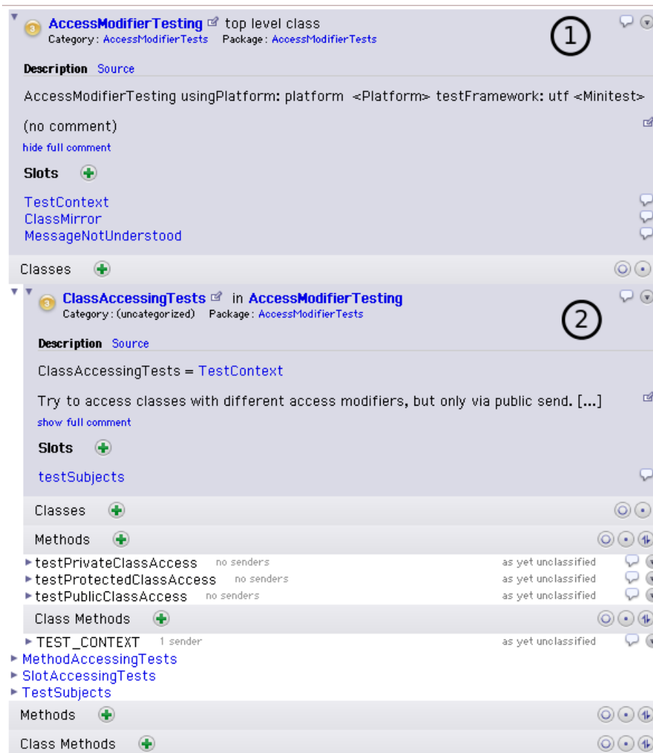
Figure 2.1: A screenshot of the Hopscotch development environment. The view of the AccessModifierTesting top-level class ① and its nested class ClassAccessingTests ② can be seen. Both within the same window and complete with documentation, slots, and methods.
