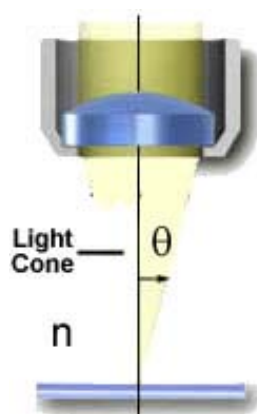
Fig 2.7: Numerical aperture (NA) of an optical device (picture adapted from [68])
