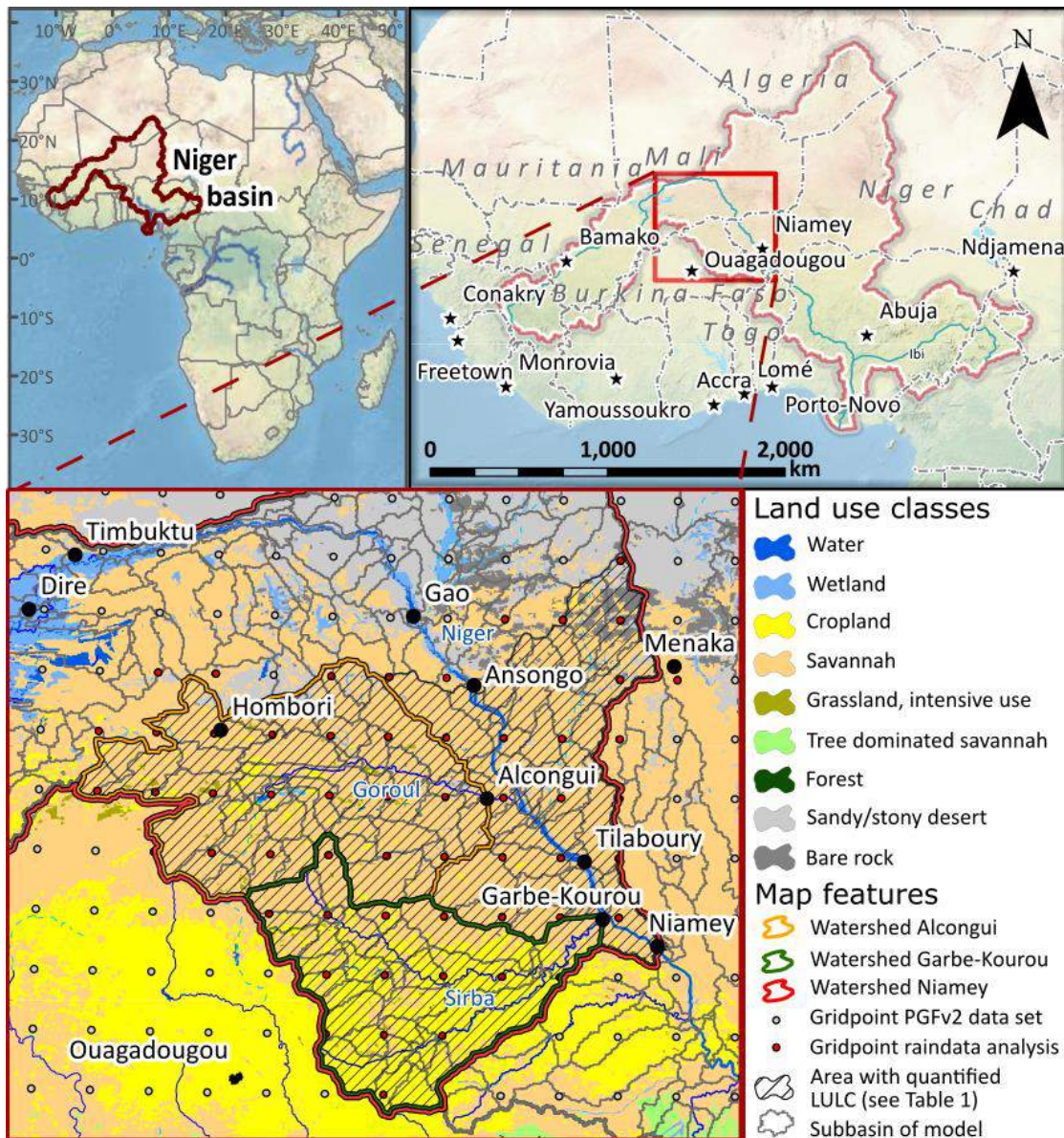
Figure 26 Map of the research area in West Africa including land use classes used in the model as base map in the year 2000. The orange, green, and red outlines mark the watershed of the gauging stations Alcongui (Goroul River), Garbe-Kourou (Sirba River) and the watershed of Niamey (Niger River). The grey dots show the grid of the PGFv2 climate reanalysis data set. The red dots show the grid of the climate data used for the analysis. The hatched area marks the region which is used for the quantification of land use and land cover changes
