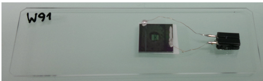
Figure 2.7: Tungsten cylinder electrode chip prepared for DEP. On this chip, all four subarrays were connected by conducting silver paint.
