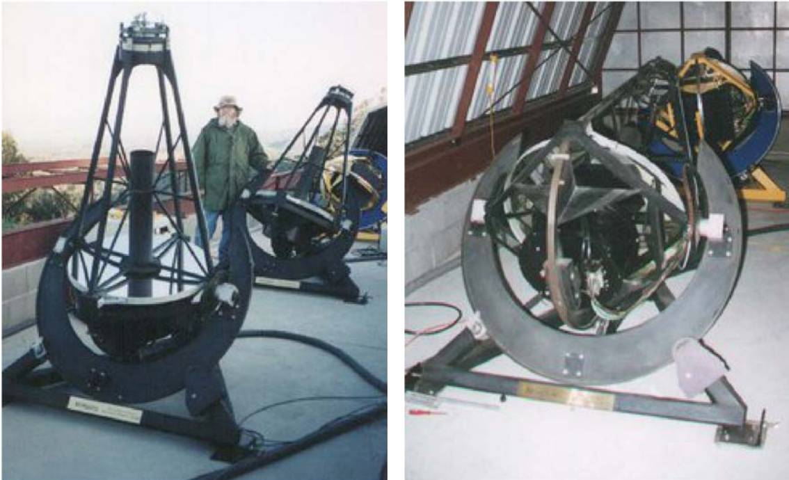
Figure 2.3: APTs at Fairborn observatory. Left: Shown are the 0.75-m APTs Wolfgang (T6) and Amadeus (T7) with T8 in the back. Right: Shown is Amadeus (T7) in the parking position with T8 in the back.
