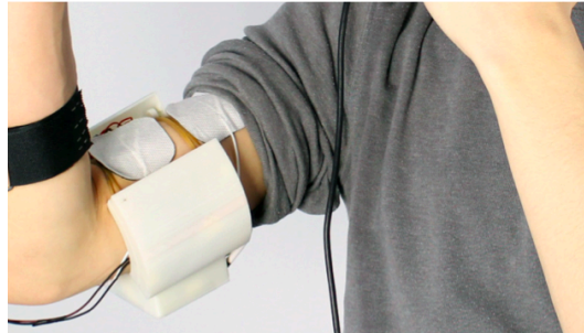
Figure 3: We show a detail of the electrical muscle stimulation component. Here, it stimulates the user's biceps brachii muscles causing an involuntary contraction that resembles force feedback.
