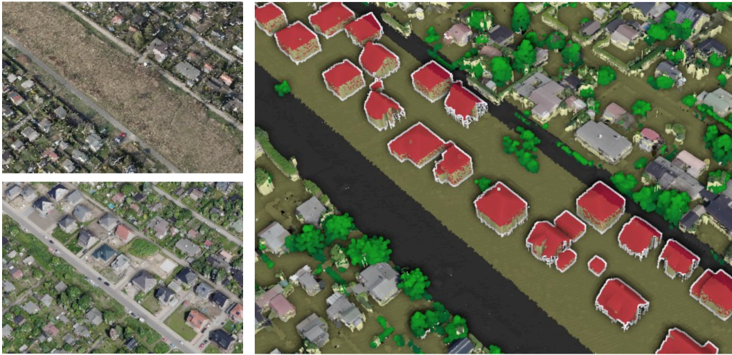
Figure 1: Multi-temporal 3D point cloud: building points that are not present in the old scan (upper left) but captured in the new scan (lower right) are highlighted with a red color scheme and by tracing their boundaries.
