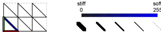
Figure 4: We map the three edges of our grid to a color channel each. The color value defines the stiffness of the corresponding beam, where the softest setting is not having the beam at all.
