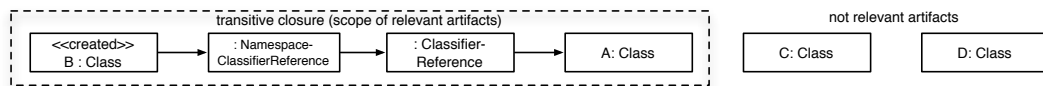
Figure 5.5.: Scope of relevant artifacts (dashed rectangle denotes scope of added class B for Generalization module)
