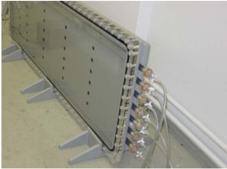
Figure B.2.: Side view on the 2D-aquifer test system with connected tubes.
