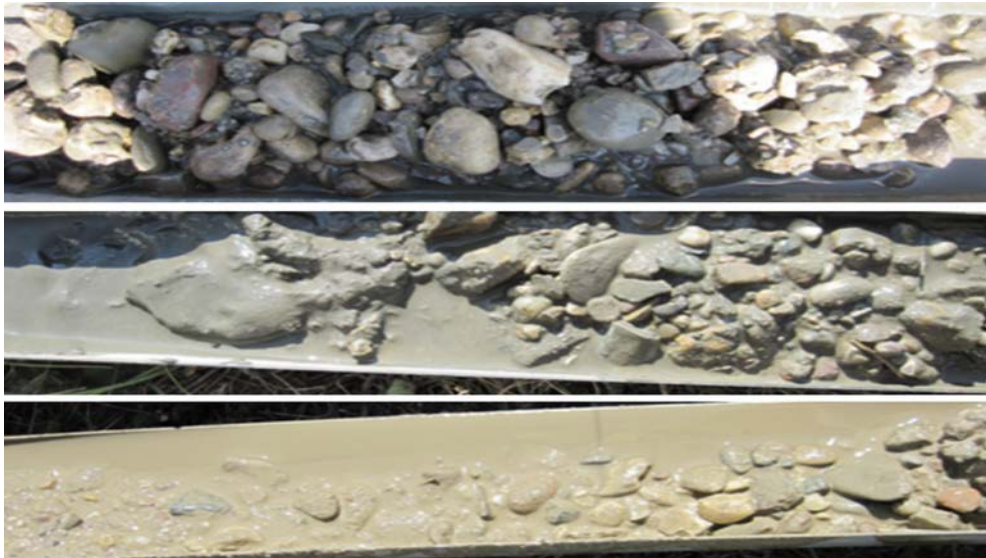
Figure 4.3.: Soil samples taken with a sonic drilling approach. The samples were all taken in a distance of approx. 50 cm downstream from the injection well. The middle image shows a sample taken in direct line from injection to extraction well. The other two images were taken 30 cm left and right from the middle sample position. All images show the core area from the gravel layer.
