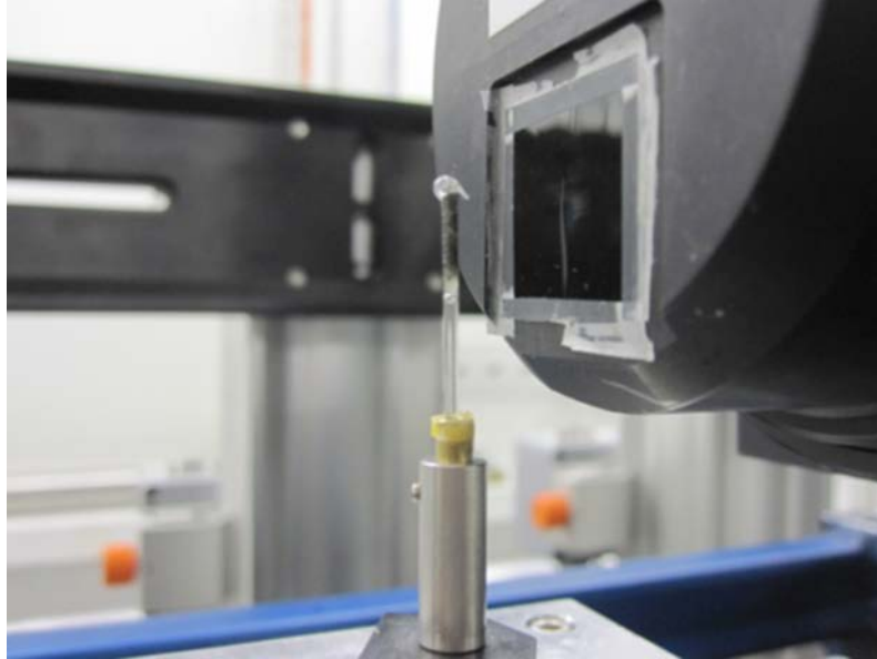
Figure 5.1.: Image of a sample positioned at the sample holder in front of the camera. The image was taken from an experiment within the set of experiments, where the presented results were obtained.
