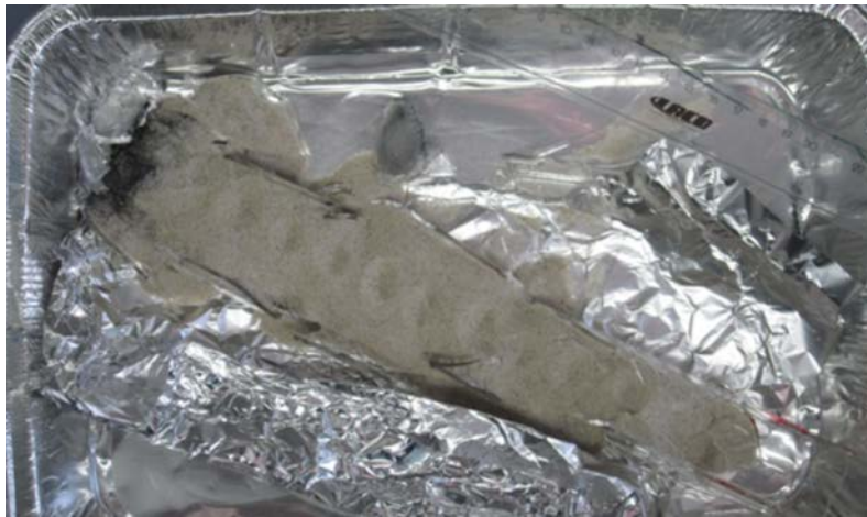
Figure B.3.: Image of the opened column. On the left side, residues of c-nZVI are visible (black color).
