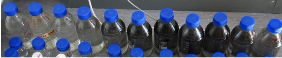
Figure 4.5.: Image of samples from the field experiment. The bottles in the upper line show images of samples taken every 30 minutes for the first five hours of the experiment (with increasing time from left to right). Beyond five hours the water samples start to lose the black color of the CIC until they are clear again (samples not shown here).
