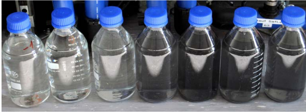
Figure C.6.: An additional image of samples from the extraction well. The tree bottles on the left side represent samples from one hour before the injection to one hour after injection. The samples on the right side represent samples taken after two hours.
