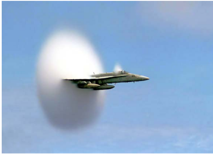
Figure 2.6: A supersonic aircraft compresses the air in front of it, which forms a bow shock. 31
