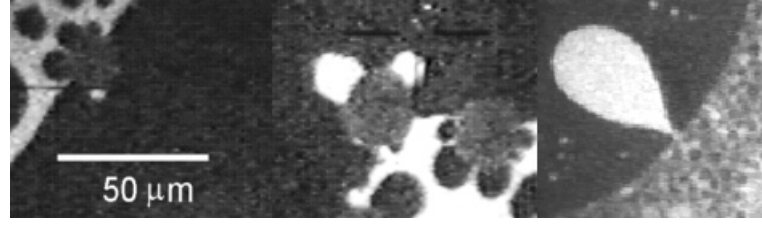
Figure 6.2.2: Droplets observed using fluorescence microscopy in the three phase coexistence region of a methyl octadecanoate monolayer (LE: bright, G: black, LC: gray) with different droplet areas A = 8.9 \times 10^{-10} \text{m}^2 , 2.0 \times 10^{-10} \text{m}^2 , 0.7 \times 10^{-10} \text{m}^2 and 0.1 \times 10^{-10} \text{m}^2 . The droplet shapes depend on their size.
