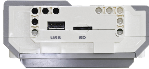
Figure 3.2: EV3 left side with host USB and microSD slot.
