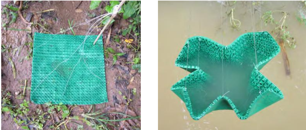
Figure 2.3: The sediment trap design, strength and balance test. Left: a fixed trap on the ground, right: bowl-shape trap when pulled up.
