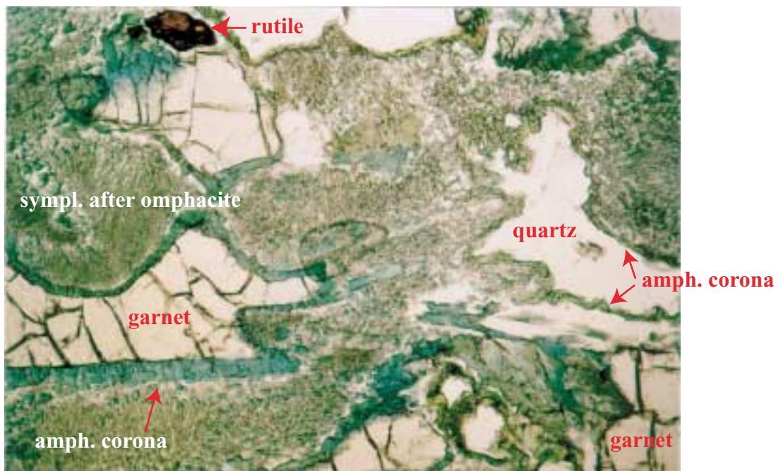
Figure 24: Photomicrograph showing amphibole coronas around garnet and quartz, indicating that coesite/quartz was present in the matrix prior to amphibole growth. Gneissic eclogite sample Dab 99101, PPL, long side is 3.6 mm.
