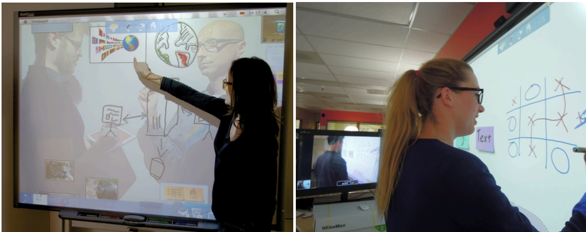
Figure 3.9: Tele-Board’s remote location setups. Left, the transparent whiteboard client is on top of a video conference in fullscreen. In the side-by-side setup (right), the video conference is on an extra display orthogonal to the Tele-Board whiteboard client.
