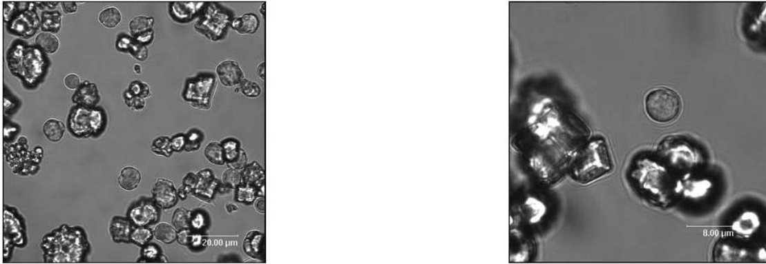
Figure 4.3.7 Confocal images of (PAH/PSS) 4 capsules from CaCO 3 cores with encapsulated PNIPAM
