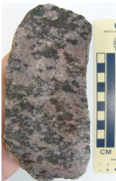
Figure A3.1: Sample HI-14 with gneissic texture macroscopically comprising of plagioclase (bright) and pyroxene (dark).
