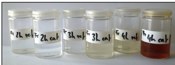
Figure 3-18: Comparison of HTC products from fructose with and without the addition of borax after different reaction times. Shown are results from 20 ml glucose solutions (30 %) with (cat.) and without (ref.) the addition of 500 mg of borax for 1, 2, 3 and 4 hours at 140 °C.
