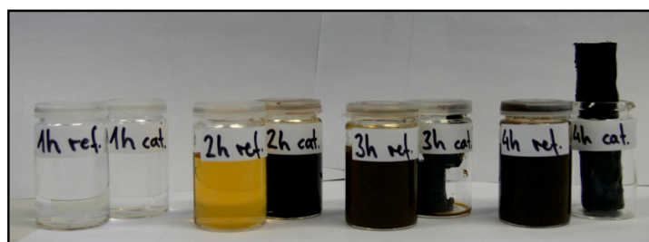
Figure 3-17: Comparison of HTC products from glucose with and without the addition of borax after different reaction times. Shown are results from 20 ml glucose solutions (30 %) with (cat.) and without (ref.) the addition of 500 mg of borax for 1, 2, 3 and 4 hours at 200 °C (reproduced from reference [67])
