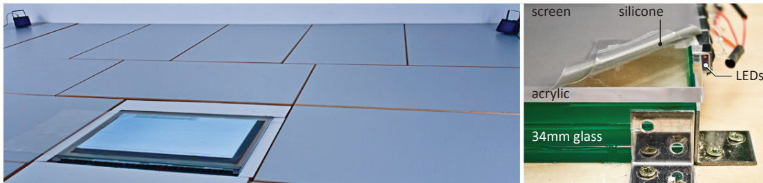
Figure 6.5: Left: Our first working prototype was composed of multiple tables. Only a sub-region of one table was interactive. (In the picture, the projection screen and compliant surface is not shown.) Right: Our prototype measures \frac{1}{2}m^2 and uses 34 mm safety glass, 8 mm acrylic, Tectosil 185 silicone, and a Rosco projection screen.
