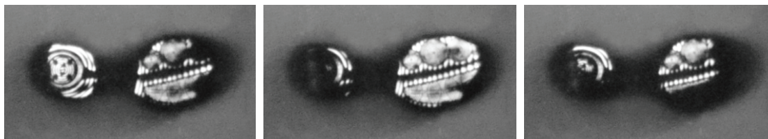
Figure 6.9: The FTIR contact area changes as the user changes posture over time.
