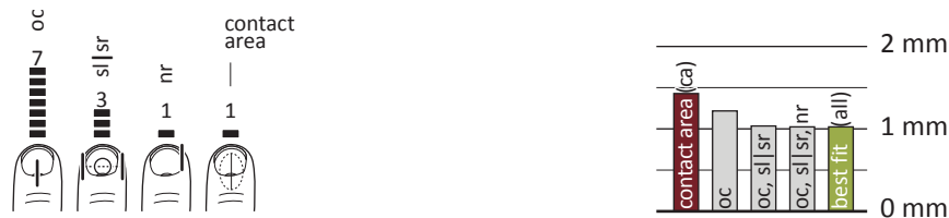
Figure 4.13: Left: Number of times each of the horizontal models produced the lowest-error offsets per participant. Right: The average error produced by the horizontal best-fit models sinks to 72% compared to CONTACT AREA. The three horizontal half models oc, sl|sr, and t|b alone account for this improvement.
