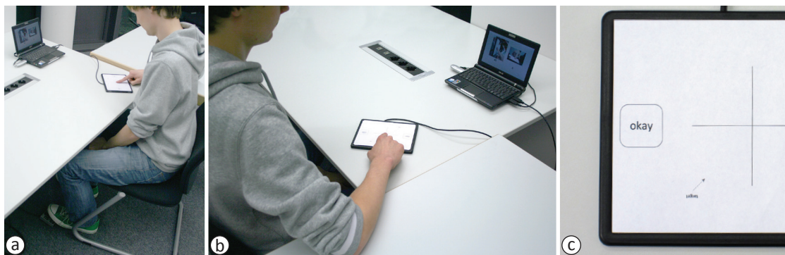
Figure 3.3: (a) A participant acquiring the crosshairs in the touchpad during the study. The laptop displays instructions and the finger orientation for the current trial. Participants committed each trial by pushing the foot switch. (b) Participants rested their elbow on the table to prevent fatigue. (c) The crosshairs mark the target.
