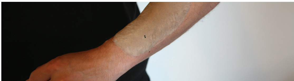
Figure 8.14: Artificial skin, created from silicone, covered the zin3out device to simulate implantation and allow for testing.
