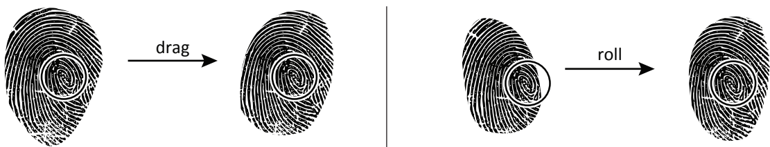
Figure 3.9: (a) When dragging, fingerprint outline and features move in synchrony. (b) When rolling the finger on the surface, fingerprint features remain stationary.
