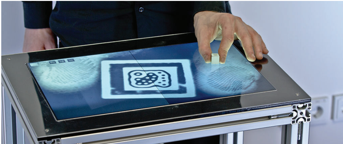
Figure 5.19: Fiberio recognizes touch, but also hovering objects (here fingers) as well as fiducial markers. This reactTivision fiducial marker [79] measures 3\text{ mm} \times 3\text{ mm} .
