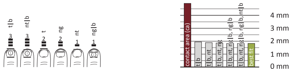
Figure 4.9: Left: Number of participants for which each vertical half model produced the lowest error. Right: Error produced when using only a subset of the half models to analyze participants. Switching from the model CONTACT AREA to T|B reduces error offsets to 44%; using all models listed on the left side reduces the error to 37% compared to the CONTACT AREA MODEL.
