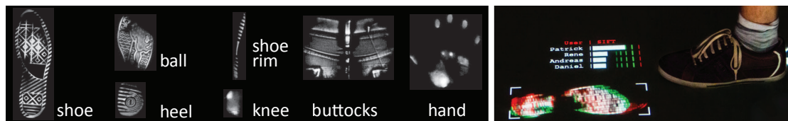
Figure 6.24: Left: GravitySpace assigns each pressure cluster the probability of being one of these contact types. Right: GravitySpace uses Harris corner detection and SIFT to match detected shoe prints against a database of registered users.
