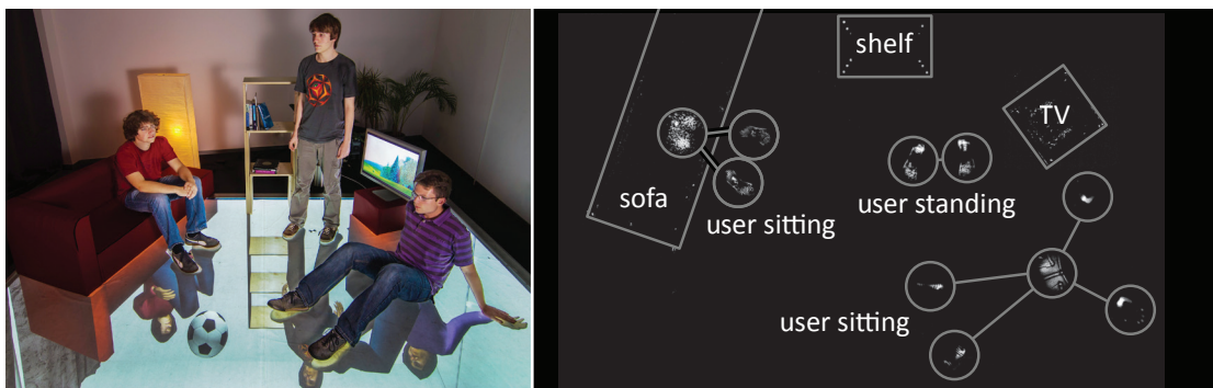
Figure 6.1: 3D reconstruction from 2D touch contacts extended to large multitouch floors. Left: Our prototype recognizes input from three users and three pieces of furniture solely in the form of 2D high-resolution per-pixel pressure sensing in the floor. Right: From the sensed 2D pressure image, we reconstruct an understanding of the physical 3D world: the position and orientation of multiple users, the identity of users in the form of personalized avatars and users' 3D body poses. The system displays a mirrored representation of this understanding on the floor (left).
