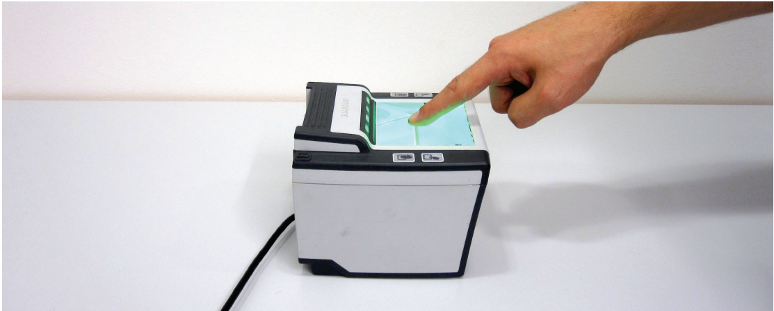
Figure 3.8: Our Ridgepad prototype is based on an L SCAN Guardian fingerprint scanner.
