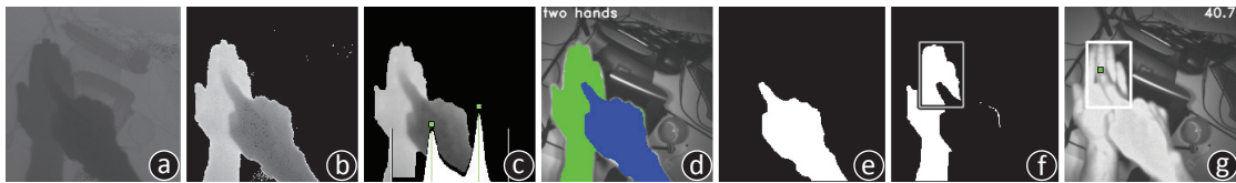
Figure 4.19: (a) In processing the raw depth image, our system (b) thresholds the image and (c) calculates a depth histogram to (d) segment the image into two masks: (e) pointing hand and (f) reference hand. From that we calculate (g) the final touch position and reference frame. This location is then forwarded to the physical device.
