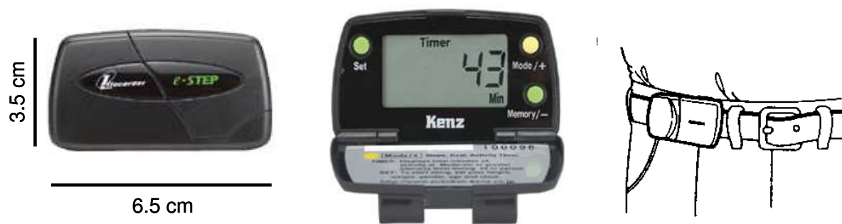
Figure 3. Kenz Lifecorder e-step pedometer – its size and position close to the hip.
