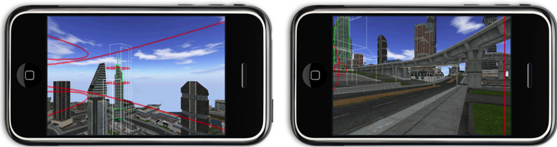
(a) An object-space 3D Halo Circle visualization combined with occlusion management showing three landmarks. One landmark is on the left front side out-of-view. One landmark is farther away on the left side out-of-view and slightly behind the camera. One landmark is right in front but occluded by another building (which is therefore rendered as wire-frame).
