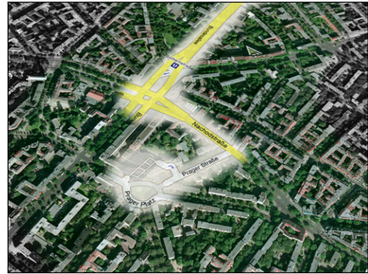
Figure 1.6: Two 2D surface lenses that combine different raster layers along a route.
