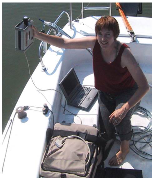
Figure 4.8: Downwelling irradiance measurements at Lake Wannsee (Germany). These were undertaken simultaneously with an HYMAP airborne scanner overflight (July 2003).
