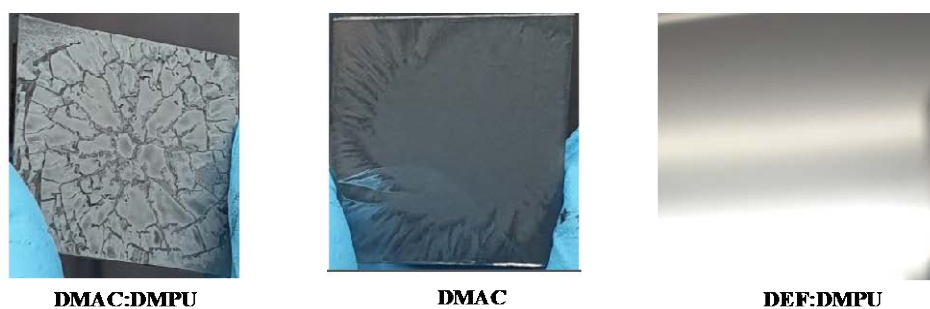
Figure A1.6: different crystallization forms of different solvents
