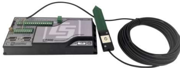
Figure 3.4: Truebner SMT 100 TDR-FDR probe connected with a Campbell CR800 data logger.
