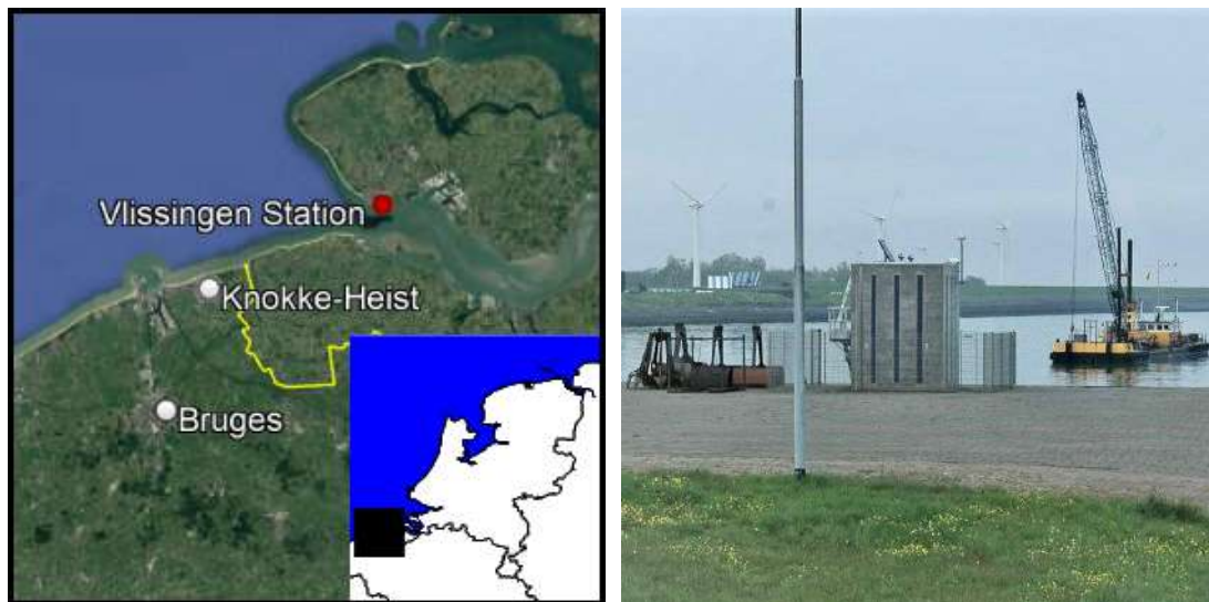
Figure 6.1: Left: Bird's eye view of the wider area of Vlissingen, the Netherlands. The yellow line denotes international borders, and the white dots show the major cities. The position of the station is highlighted with a red dot (Acquired from Google Earth 1 ). Right: GNSS antenna installed in the marina, on a 6.5 m monument (Viewing angle in the southeast direction, rendered from Royal Observatory of Belgium 2 ).
