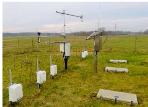
Figure 5.5: Cosmic-ray sensor installed in Füstensee station. The device is some metres away from the GNSS receivers (Looking angle in the south direction).
