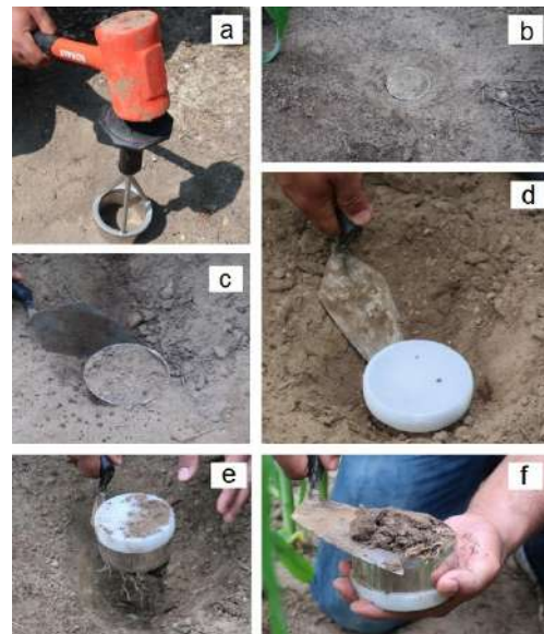
Figure 3.3: Soil-sampling process. A metal case is inserted in the soil, and it is extracted smoothly in order not to destroy the natural structure of the sample. Next, the surface is flattened to align with the ring's lower and upper edges (Reprinted from Shokrana and Ghane 2020).
