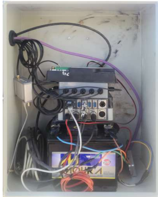
Figure 7.3: Equipment assembly of the station in Pozuelos. The instrumentation includes a TDR-FDR logger, a computer, a Javad Delta TRE-G3T multi-frequency and multi-constellation geodetic receiver, a battery (top to bottom order), a Geostar GeoS-5M low-cost receiver (top left), and a solar charge controller (bottom right).
