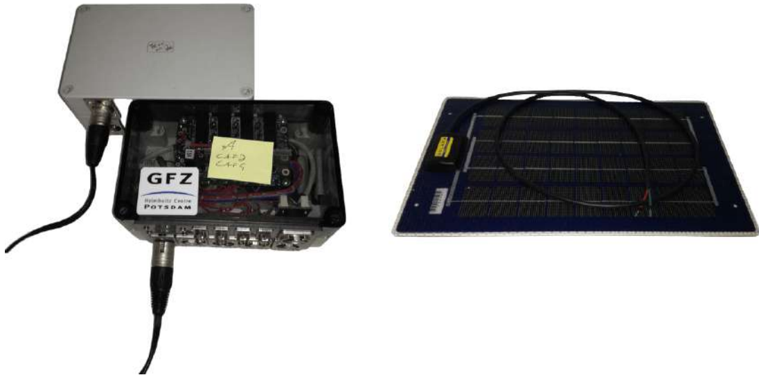
Figure A.1: Left: TinyPc Linux-based computer connected to a portable battery. Right: SOLARA 100 Wp solar panel. The computer was used for the transmission of commands to the sensors to ensure their uninterrupted operation and for data storage. The solar panels were only used in the case there was not possibility for connection to the local network.
