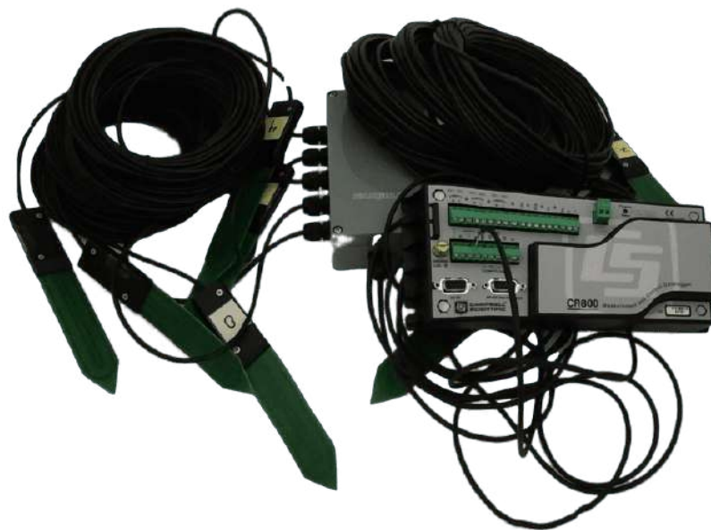
Figure A.5: Campbell CR800 data logger connected to nine Truebner SMT-100 soil-moisture probes. The data logger includes a processor that controls the probes and stores the observations. The measurements are obtained by the probes that are buried in the soil.
