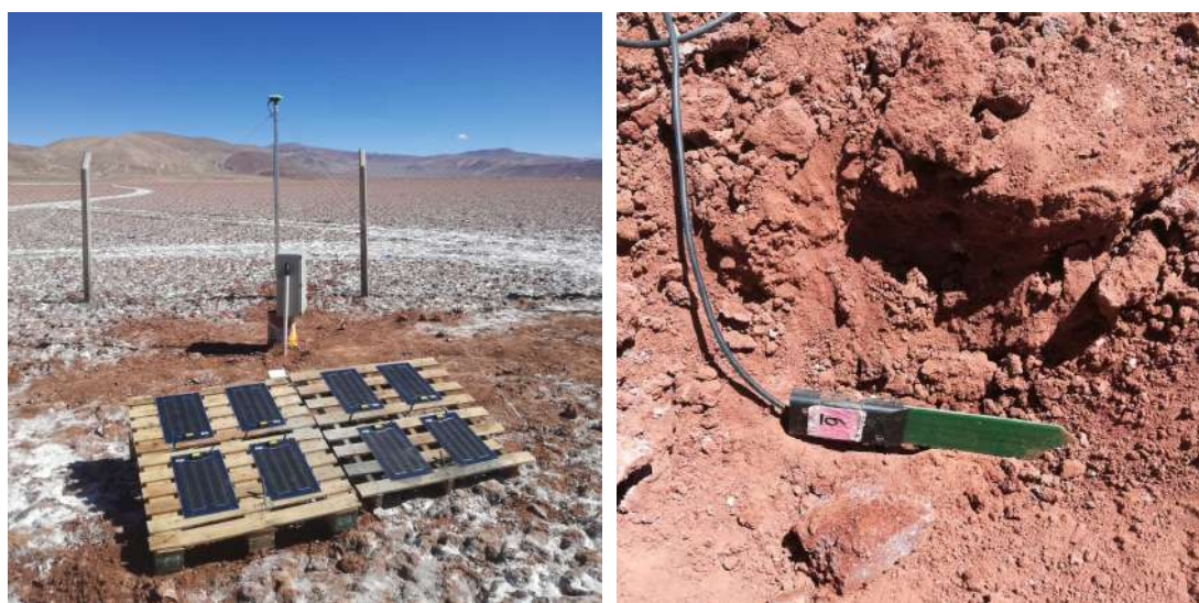
Figure 7.6: Pozuelos station. Left: Detailed overview of the base, where the GNSS is installed along with additional sensors, used for the mining operations. The antenna is attached on a 2.5 m pole, the solar panels are installed for energy supply, and the metal box includes all necessary instrumentation (Looking angle in the southeast direction). Right: Soil vertical profile and a TDR-FDR probe placed at 10 cm depth. In the photo are shown the soil granules, as well as the formatted rock salts.
