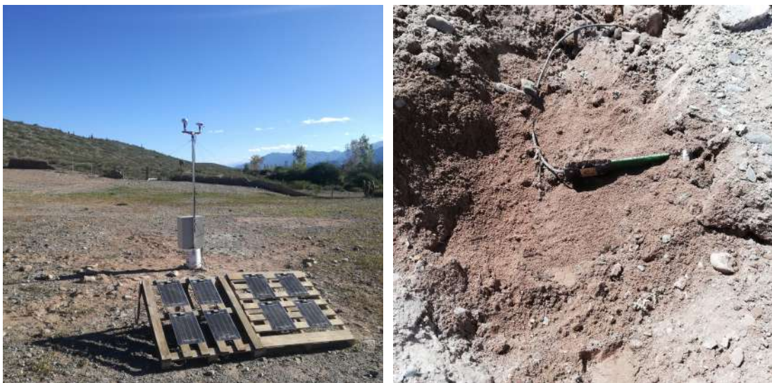
Figure 7.5: Payogasta station. Left: GNSS antennas attached on a 2.5 m pole, as well as solar panels installed for energy supply. The metal box includes all necessary instrumentation (Looking angle in the southeast direction). Right: Soil vertical profile and a TDR-FDR probe placed at 5 cm depth. The development level of the soil is comparable with Tolombon station (cf. Figure 7.4).
