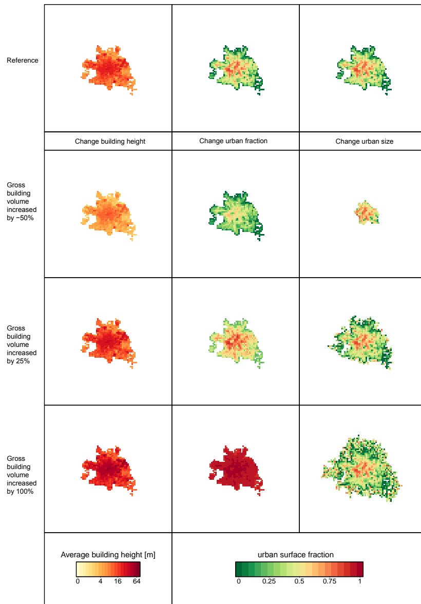
Figure B.5: Visualization of some urban canopy parameters (UCP) datasets from different urbanization scenarios based on the UCP dataset of Berlin. The first column shows the average building height map, the second and third show the urban surface fraction maps, respectively. Panels in the first row are from real UCP dataset of Berlin used in the reference run, whereas Panels in other rows are from UCP datasets where gross building volume is increased by -50%, +25%, and +100%.
