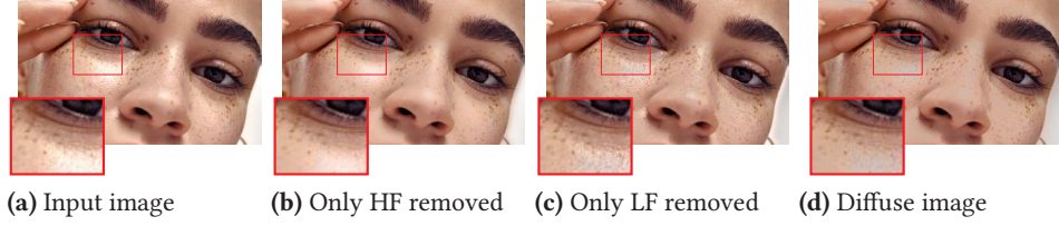
Figure 3.5: Effect of high frequency (HF) and low frequency (LF) specularity removal on an input image. For the resultant diffuse image Fig. 3.5d we remove both HF and LF specularities.
