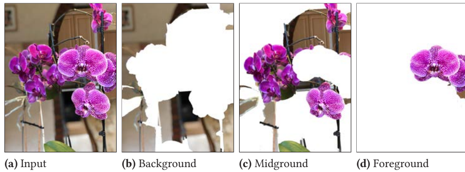
Figure 5.6: Example visualization of separating an input image (a) into individual LDI layers (b)-(d), based on quantized depth data (Fig. 5.5c). White indicates pixels associated to other layers.
