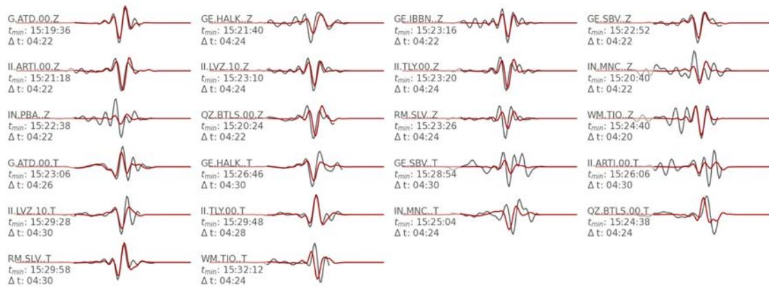
Figure S6. Waveform fits of the mean model (red) and observed data (black) from full MT inversion of earthquake C1. Channel information, start time of each trace and length of the given traces are given left of each trace.
