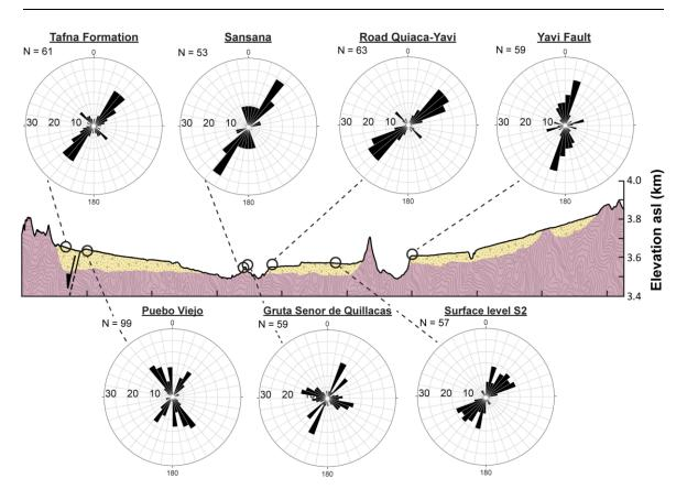
**Figure 30:** Rose diagrams of joint orientations at different sites along an E-W profile crossing the basin (for location see Figure 2). Main orientation of the joints is NE-SW to NNW-SSE. A small amount of secondary joints was measured in (sub-) perpendicular direction. Tensional stress is inferred to be oriented NW-SE to E-W perpendicular to the orientation of the joints.
