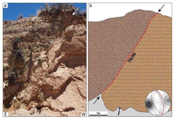
**Figure 28:** Major displacement at the southern outcrop at the sand pit East of Yavi. Conglomerates in the East are offset along a E-dipping fault plane for a cumulative count of at least 5 m. **a**) Outcrop picture, fault plane indicated by white arrows. **b**) Graphic interpretation of the outcrop, fault plane displayed by black arrows, hammer for scale.
