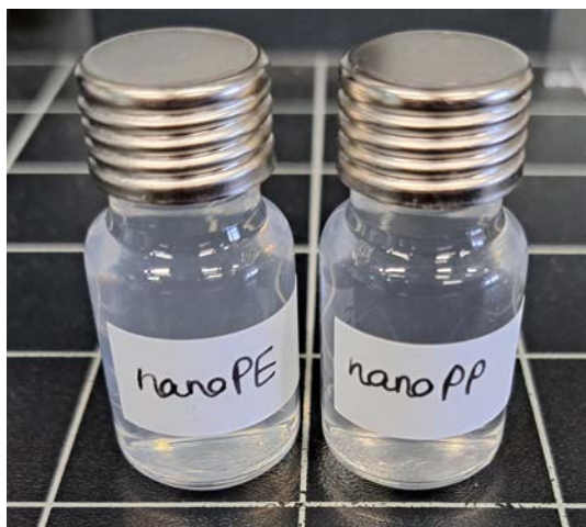
Figure 3.1: Photograph of the dispersions of nanoPE (left vial) and nanoPP (right vial) prepared under the conditions given in Table 3.2. The dispersion of the nanoPE particles is more turbid than the dispersion of nanoPP, which is due to the higher concentration and aggregates formed.
