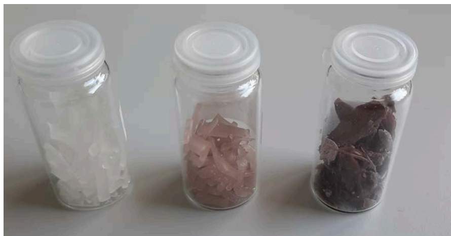
Figure 3.9: Photograph of the PP with increasing gold content. Left: pure PP prepared without gold salt; Centre: PP with a gold content of 0.1% gold; Right: PP with a gold content of 0.5% gold.
