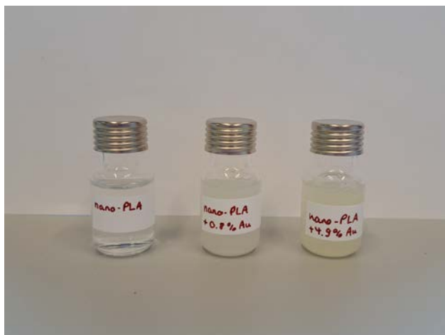
Figure 3.23: Photograph of the samples dispersed in water. Left: nanoPLA without gold. Middle: nanoPLA with 0.8% Au. Right: nanoPLA with 4.9% Au. All samples have a PLA concentration of c_{\text{PLA}} = 1.0 \cdot 10^{-3} \text{ g mL}^{-1} .
