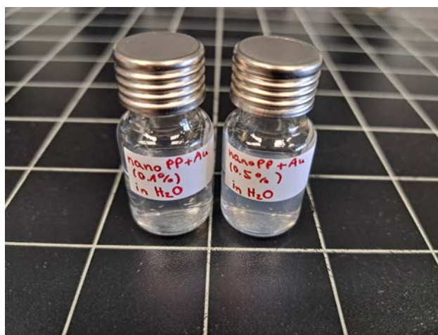
Figure 3.12: Photograph of vials containing the gold-stained nanoPP particles dispersed in water. Left: NanoPP dispersion prepared with the PP containing 0.1% gold. Right: NanoPP dispersion prepared with the PP containing 0.5% gold.
