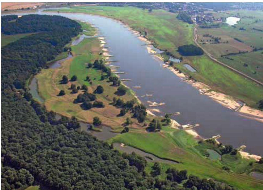
PHOTO 14.3 The Elbe near the village of Cumlosen (upper right) at Rkm 467–470. The lowland section of the river channel is nearly totally fixed by perpendicular groynes made of stones. On the left bank some broken groynes may be seen, which are less filled with sediment deposits than others. Ancient river channels are visible on the left and right banks; the left side has a hardwood floodplain forest (Photo: Federal Institute of Hydrology).
