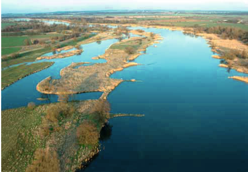
PHOTO 14.4 The Oder River downstream of the city of Frankfurt. The straightened river channel is fixed by perpendicular groynes and ancient river channels are visible. The river corridor, which is bordered by dikes, has only sparse tree cover because the trees suffer from ice drift that may occur during high water levels in winter (Photo: Oder-Luftbild, Lebus).
