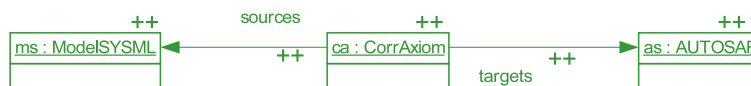
Figure 8: Axiom of the triple graph grammar for the transformation from SysML to AUTOSAR
