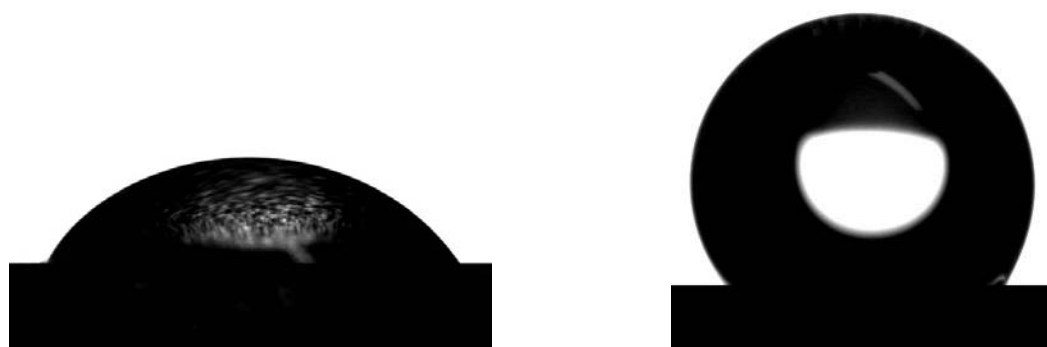
Fig.33. Contact angle on aluminium alloy plates after the standard cleaning procedure (left) and after treatment (right) with solution of alkoxy silanes in DEPh (the composition of the mixture is the same as the core of the microcontainers).
