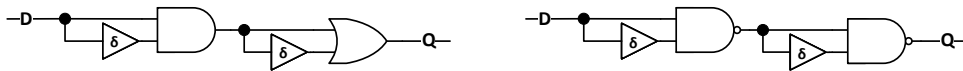
Figure 5.2: Proposed pure standard cell-based transient filter cells: (a) AND-OR-based, (b) the NAND-based optimization
